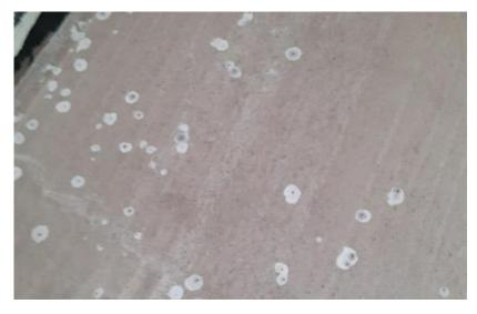
Although this problem is merely cosmetic, surface repairable and will have no effect on compressive strength or thermal properties it is better avoided.
